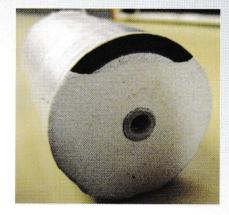
Thin polypropylene films wound with a high tension are particularly prone to mechanical stress at the margin side. Damage can then easily occur on the adjacent metal layer. A wave-cut at the free margin edge spreads these stresses and reduces the risk at high operating temperatures or high currents.
